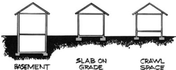
For instance, it is common to have a basement under part of the house and to have a slab-on-grade or crawlspace under the rest of the house. In these situations a combination of radon reduction techniques may be needed to reduce radon levels to below 4 pCi/L.
